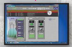
Use any of the connection methods to transfer the PUMP Vision and MOTOR Vision data into SCADA Vision. Or use your existing SCADA system. Connect with a variety of protocols including Modbus IP, DDE, and OPC.
